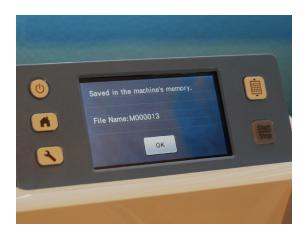
**Step 5. Prepare your fabric:** On the ScanNCut machine, press the "Wrench" button on the far left to show you the settings. Set the "Cut Speed" to "1" and the "Cut Pressure" to "5."
